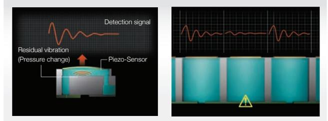
The piezo element (sensor) detects the residual vibration (pressure change) in the ink chamber and diagnoses the nozzle condition.
